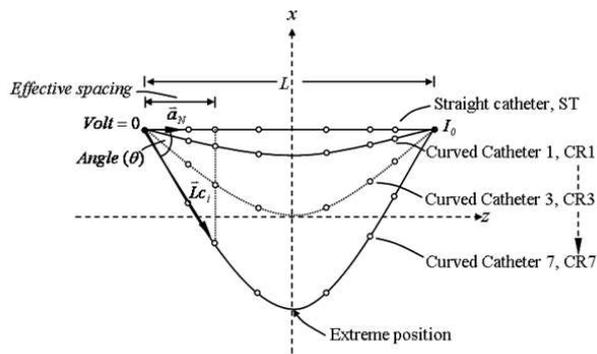
**Fig.2:** Configurations of conductance catheter curvature (the example shows 6 measurement electrodes)
