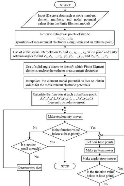
Fig. 5: The Pattern Search Algorithm method used for optimizing percent true volume error ( $\varepsilon_t$ ) using conductance catheter techniques
