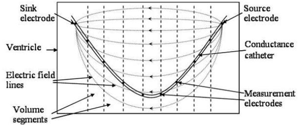
**Fig.1:** Model of a conductance catheter inserted into the model
