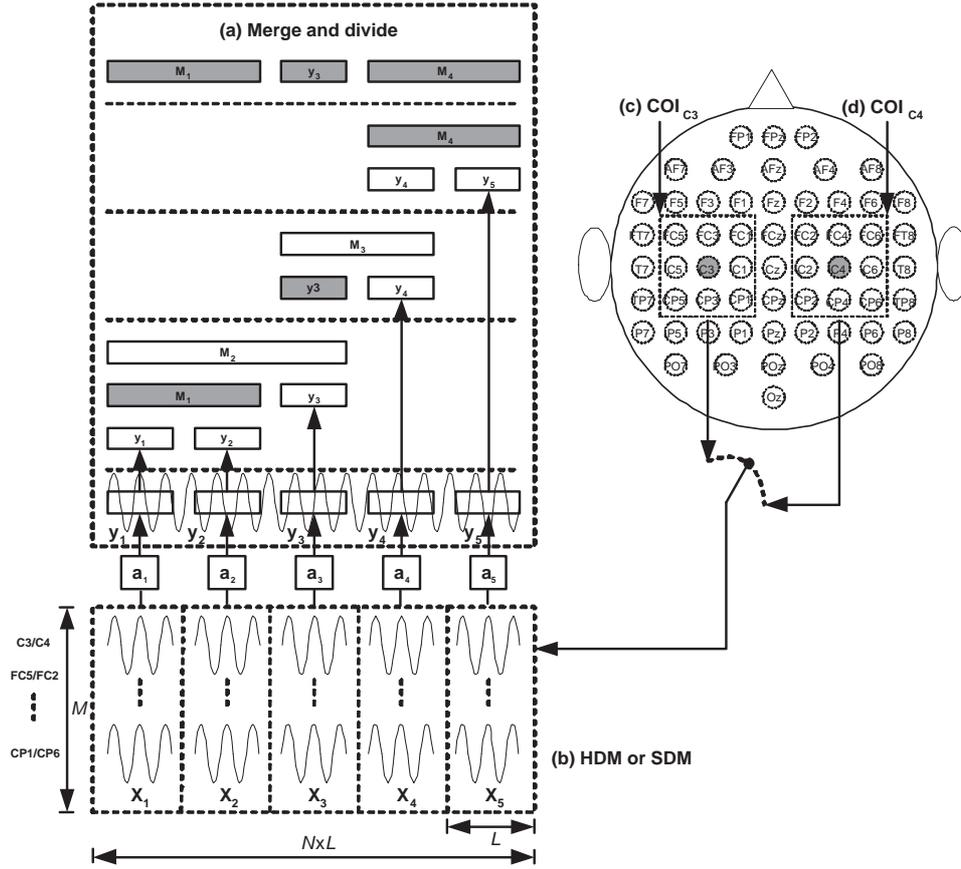
**Fig.3:** Design process of the MF-LDB: (a) merge and divide procedure, (b) HDM or SDM, (c)  $COI_{C3}$ , and (d)  $COI_{C4}$ .
