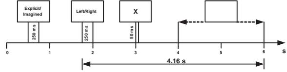
**Fig.1:** Data acquisition stage of the EEG signal used for classification
