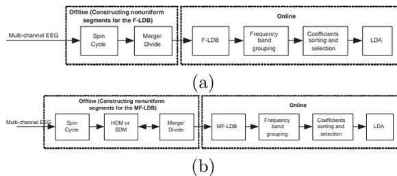
**Fig.2:** Block diagram of (a) the conventional left/right index finger movement imagery classification method [8] and (b) the proposed classification methods.
