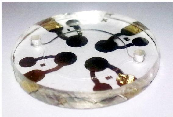
**Fig.2:** QCM sensor array with PDMS chamber
