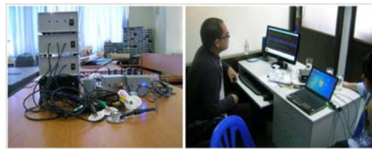
Fig.14:: ECG & HS equipment prototype with monitoring via WBBN network.
