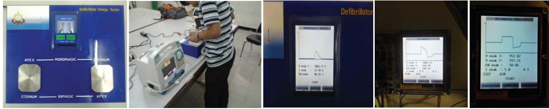
Fig.2:: Data table and graph relationship between standard energy and output voltage across resistor.
