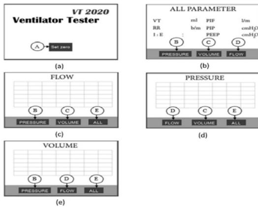
**Figure 6.** The display design (a) the 1<sup>st</sup> page when power on, (b) the all-parameter page, (c) the flow data page, (d) the pressure data page, and (e) the volume data page.
