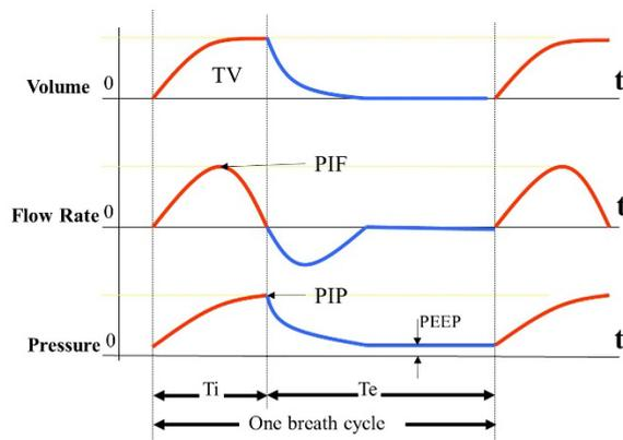
**Figure 1.** The volume /time, Flow rate/Time, and Pressure/ time graph during the breath cycle and the related parameter were shown in the graph.
