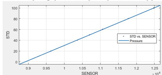
**Figure 13.** The relation of the pressure sensor data compared with the standard digital pressure gauge
