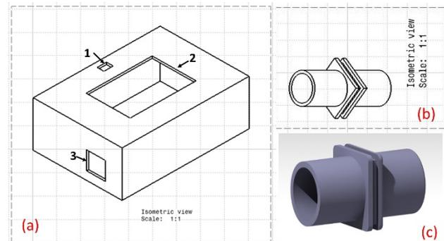
**Figure 8.** (a) the case design when (1) the on-off switch (2) the HMI display and (3) the straight pipe connectors to a ventilator, (b) the connector design, (c) the 3D connector.
