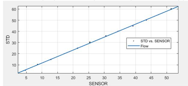
**Figure 12.** The relation graph of the flow sensor data compared with the standard flow meter
