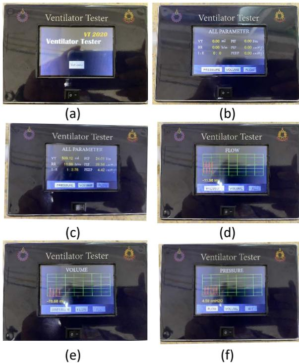
**Figure 14.** The display result (a) the 1<sup>st</sup> page when power on, (b) the all-parameter page without data, (c) the all-parameter page with data, (d) the graphical of flow data page, (e) the graphical of pressure data page, and (f) the graphical of volume data page.
