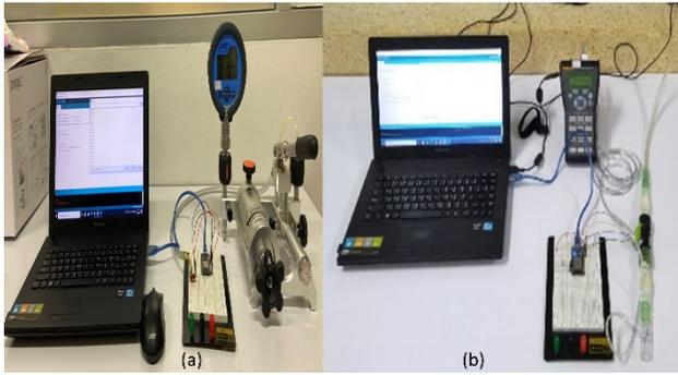
**Figure 10.** The calibration of (a) pressure and (b) flow sensors compared with the standard equipment.
