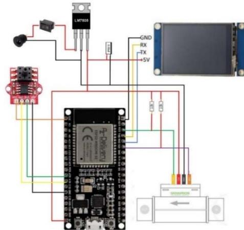
**Figure 5.** The overall circuit use in the designed prototype.
