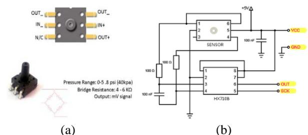
**Figure 2.** (a) Pressure sensor MPS20N0040D-S (b) The circuit diagram of pressure measurement [5]
