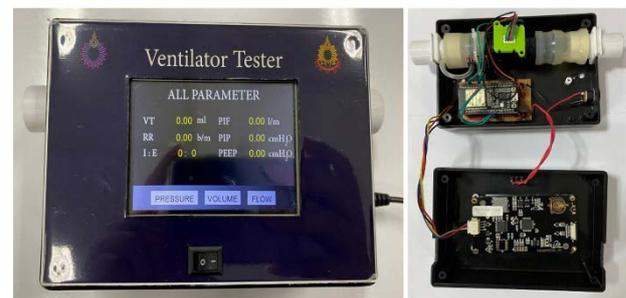
**Figure 9.** The ventilator tester prototype
